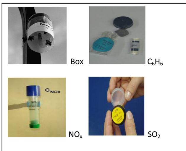
**Figure 1:** Carried box samples (Passive sensors: Passam)
